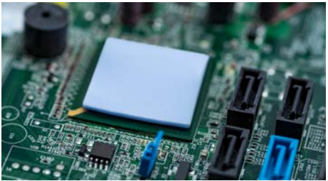
The low oil-bleeding property protects components from contamination.
