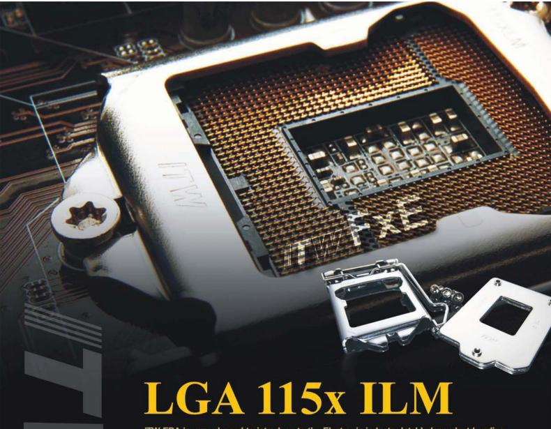
ITW EBA is very pleased to introduce to the Electronic industry Intel Independent Loading Mechanism (ILM) for Intel Socket H for both LGA 1155 & LGA 1156 (LGA115X). ILM provides the force needed to seat the 115x-LGA land package onto the socket contacts. The ILM is physically separate from the socket body. The assembly of the ILM to the board is expected to occur after wave solder. The exact assembly location is dependent on manufacturing preference and test flow.
